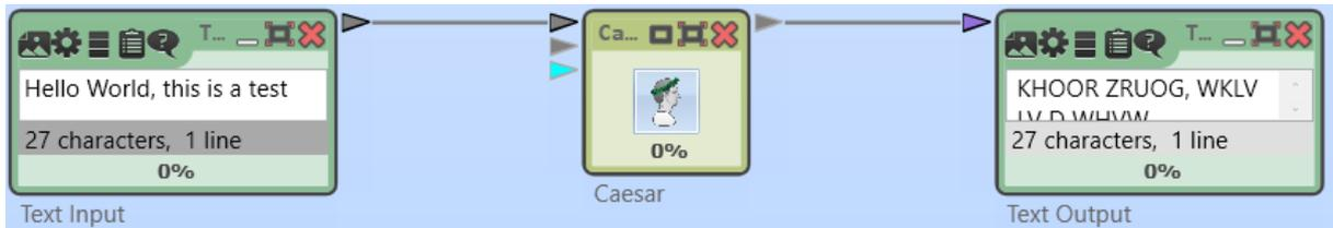
Try to type into the “Text Input” while the graphical program is being executed. CT2 will update your ciphertext in the “Text Output” component at once.
